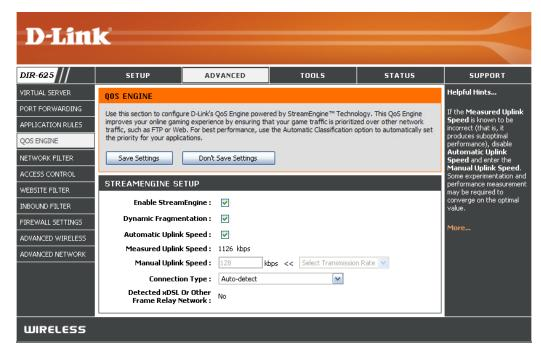
Manual Uplink The speed at which data can be transferred from the router to your ISP. This is determined by your ISP. ISP's often speed as **Speed:** a download/upload pair. For example, 1.5Mbits/284Kbits. Using this example, you would enter 284. Alternatively you can test your uplink speed with a service such as www.dslreports.com.
